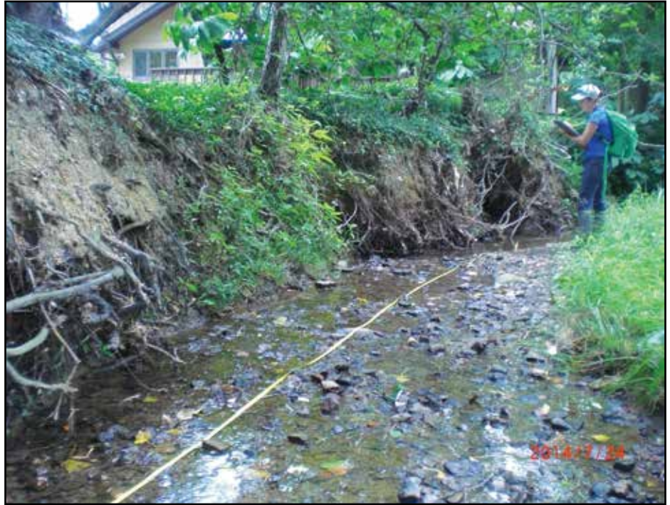
Above: Assessing streambank erosion in Baldwin Creek. Below: BEHI results are used to target individual properties for streambank stabilization assistance.
