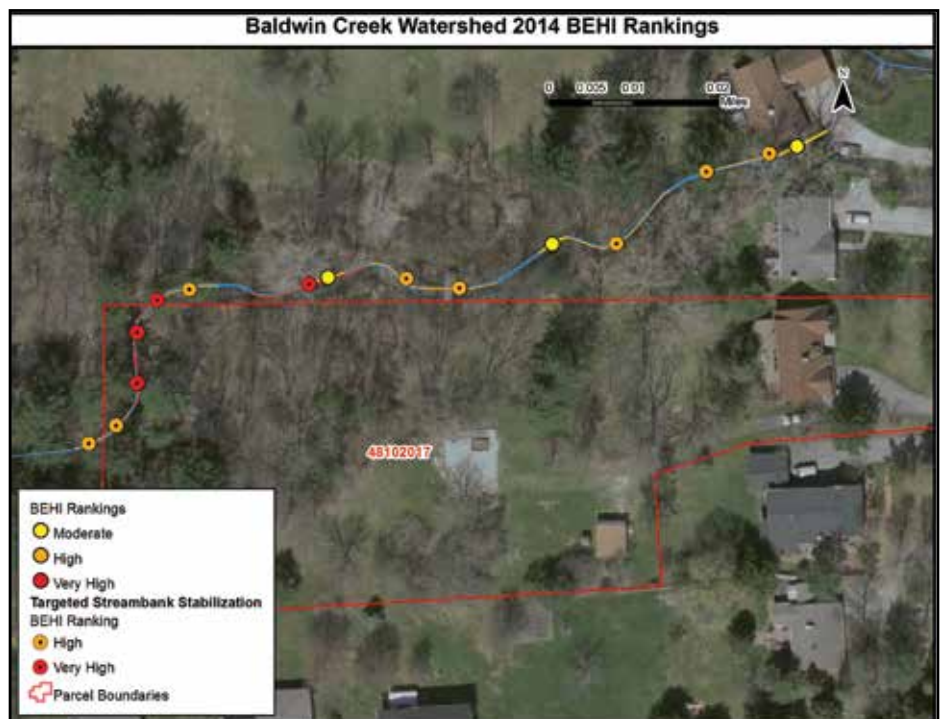
Above: Assessing streambank erosion in Baldwin Creek. Below: BEHI results are used to target individual properties for streambank stabilization assistance.
